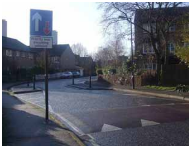
Figure 4.7 Pinch-point with priority operation
